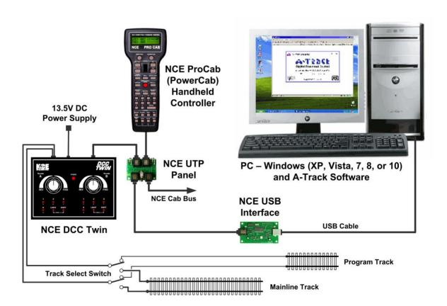
Alternatively, if you have an NCE Power Pro Command Station, you can simply connect A-Track to it via a standard Serial Port, if you have an older PC which is fitted with one, or via a USB Port and any readily-available USB-to-Serial (RS232) converter unit, as shown below –
