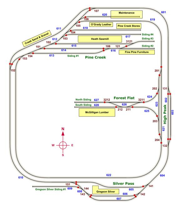
Here the **red** dots represent the track breaks which separate blocks, with the assigned block numbers (addresses) from 0601 to 0628 shown in **blue**, and turnout addresses shown in **brown**.
