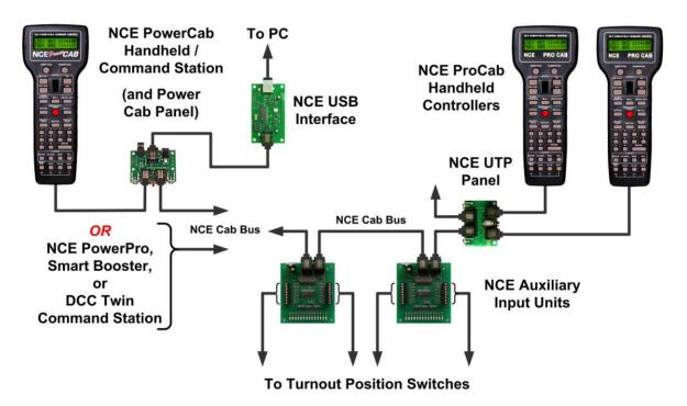
Each turnout to be monitored on the layout needs to be fitted with an electrical switch, mechanically linked directly to either the turnout throw-bar or to the turnout actuating machine (motor). Slow-motion (stall) turnout machines such as Tortoise and Cobalt already incorporate suitable switches for this purpose, but external switches generally have to be added where you are employing solenoid (snap) motors or servos to throw your turnouts.
