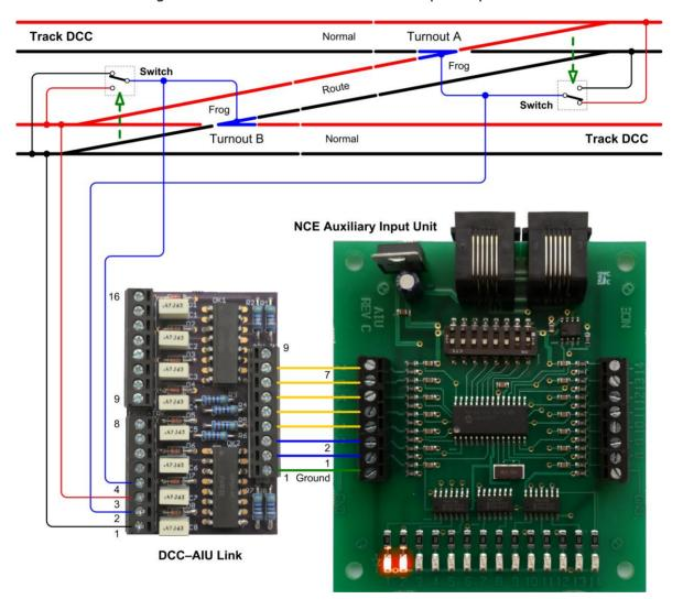
Each pair of terminals in the two 8-way terminal blocks on the left side of the DCC-AIU Link module connects to an individual turnout. A connection to the frog is taken to the
