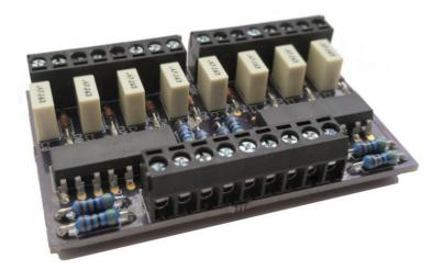
The DCC-AIU Link module allows you to connect up to eight turnout frogs to corresponding AIU inputs, without any danger of damaging the AIU, by virtue of the pair of optical isolator chips which can be seen in the centre of the module.
