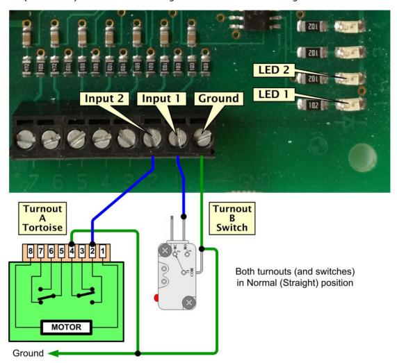
Each switch should be connected such that, when the turnout is set in the Normal (Straight) direction, the switch is open, ie. there is no connection between the common terminal (Tortoise #4 or COM) and the switch terminal connected to the AIU input (the Normally Open, Tortoise #2 or NO, contact in the examples above). In this state, the light-emitting diode (LED) associated with that AIU input will not be lit.
