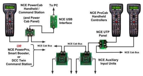
To Turnout Position Switches or Block Detectors
