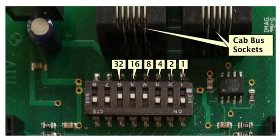
With an NCE Power Pro system, you can use any address in the range 02 to 63, although the recommendation is to restrict AIU addresses to the range of 50 to 63.
