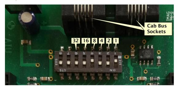
Hence, in the AIU pictured above, with switches 1 and 4 moved towards the Cab Bus sockets, the Cab Address is (1 + 8), ie. **09**.
