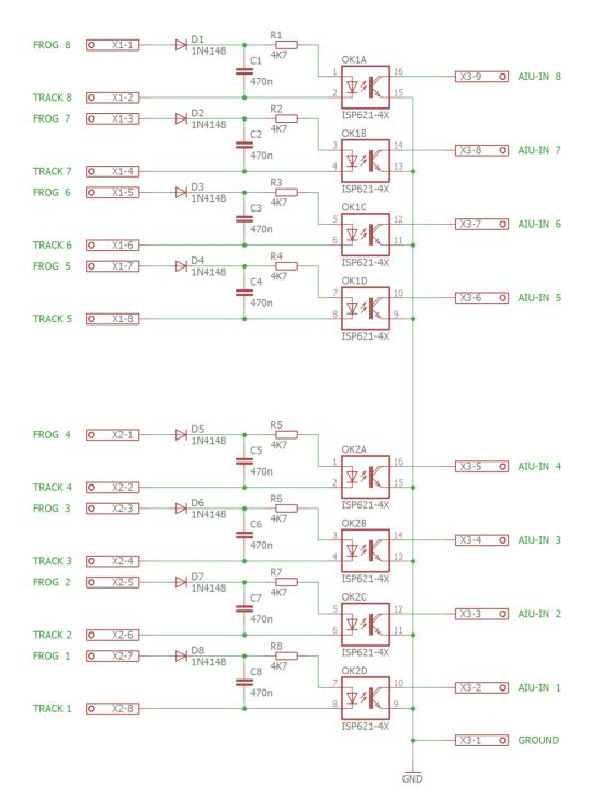
The module consists of eight independent channels. When the input terminals of a channel are connected to the DCC track voltage, as when an attached turnout is in the Route position, the input capacitor (C1 - C8) is charged via a diode (D1 - D8) to the full positive DCC voltage. This then illuminates the internal LED of the relevant section of the optocoupler (OK1A-D or OK2A-D) which in turn switches on the adjacent internal phototransistor and connects the corresponding AIU-IN output to Ground.
